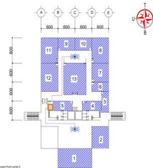
Gambar 18. Denah Keyplan AP Lantai 5
